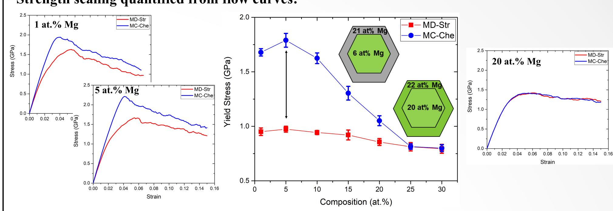
The peak difference in flow stress between the alloys occurs at the global composition where grain boundary segregation is maximized. This state corresponds to a minimum in the grain boundary energy and excess free volume, which manifests in the mechanical properties as a peak strength.
