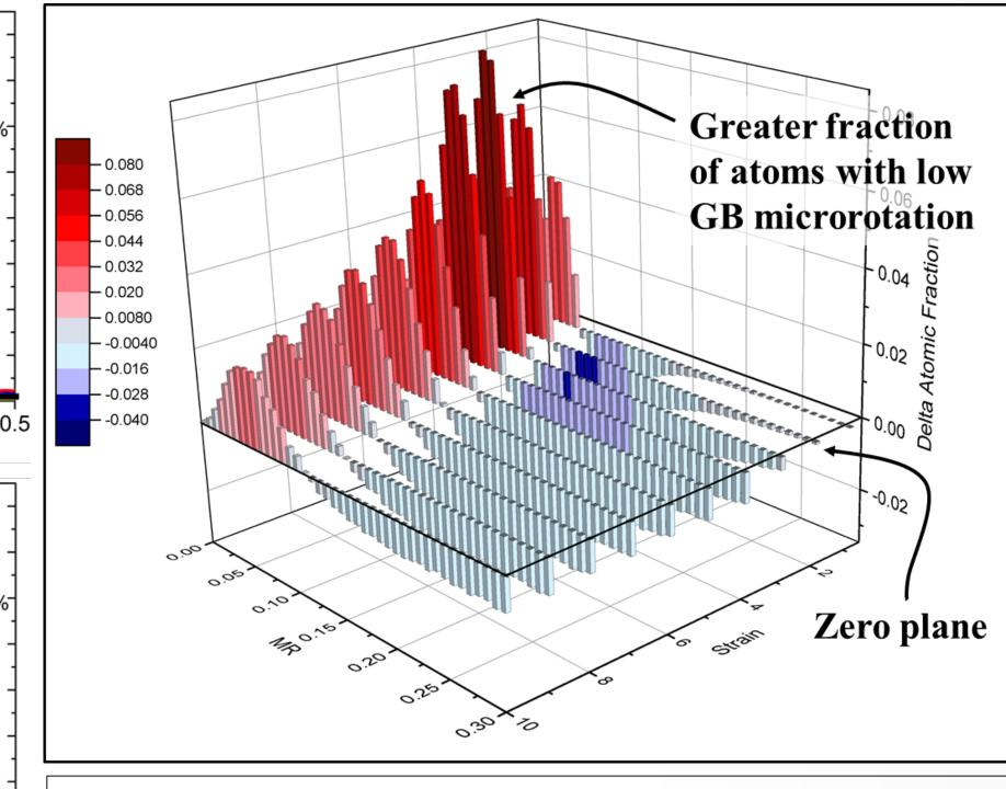
At low strains, microrotation in the GB Segregated State is reduce from the Chemically Homogenous State, indicating stabilization of the GBs.
