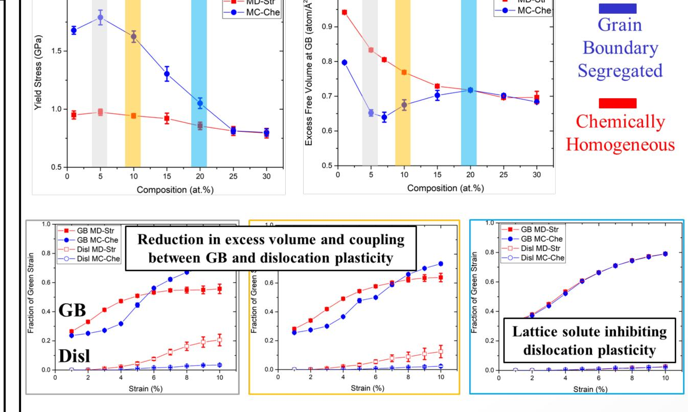
Comparing trends for the same global composition, strain accommodation by the grain boundaries is suppressed by the segregation of Mg atoms.
