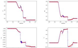
Shock tube test problem solved using 256 and 800 grid cells at  $t\,=\,0.1$  s.
