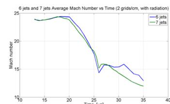
Degradation of Mach number during compression in liners obtained by merger of 6 and 7 plasma jets.
