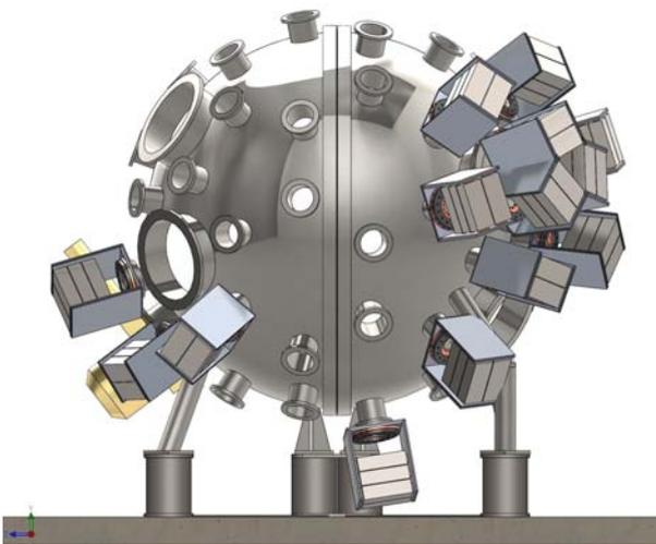
Schematic of PLX experiment under construction at LANL
