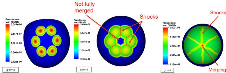
Distribution of density on spherical slices of data from 6 jet merger simulation using FronTier. Slices are selected at the leading edge of jets / liners (defined as the location of maximum average ram pressure).
