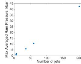
Scaling of Ram Pressure at Full Implosion
