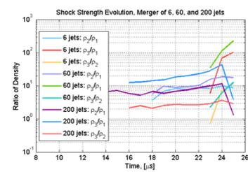
Characterization of Liner Non-uniformities: Strength of Primary and Secondary Shock Waves
