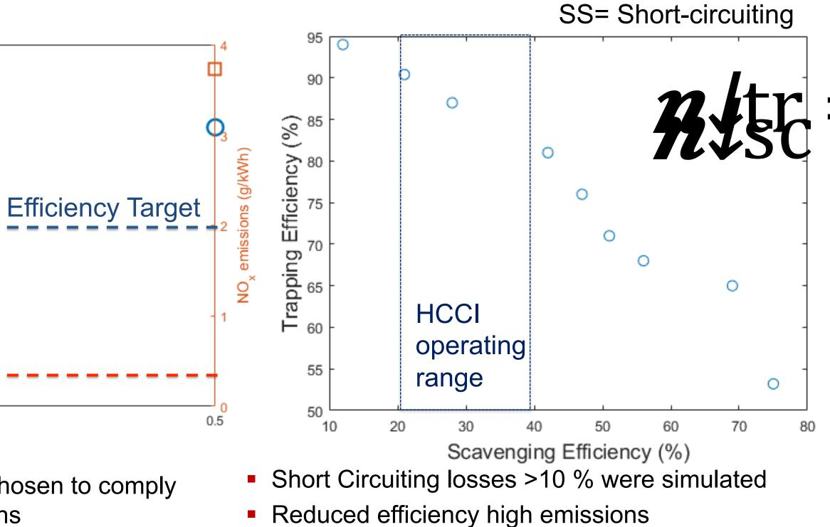
ansfer port relocation will be considered to reduce trapping inefficiency Fiston redesign to block the direct flow will be investigated
