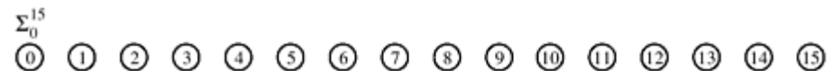
(e) Accumulation of the sum at processing element 0 after the final communication step
